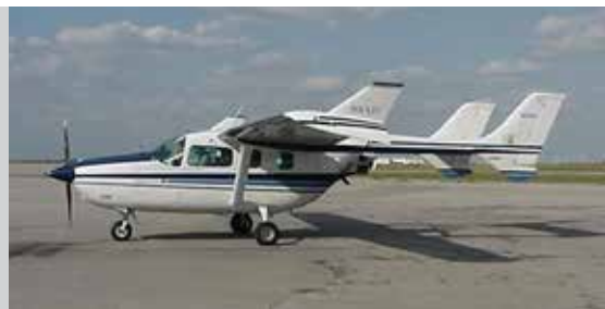
A Skymaster modified with the addition of winglets and medium-size tail boom fairings.
