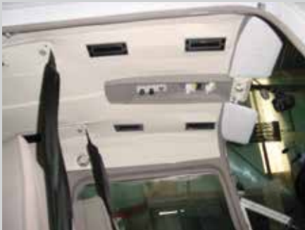
Air outlets over the passenger seats on the 1963 to 1972 models.
