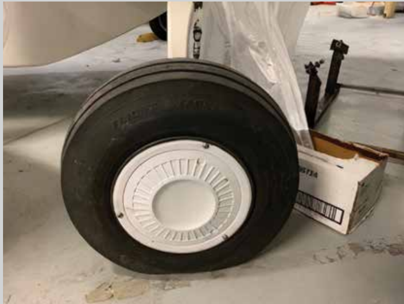
Hubcaps keep wheel bearings and seals clean.
