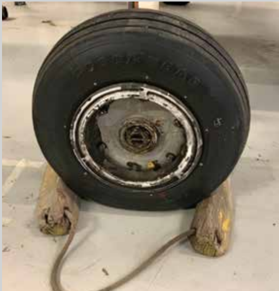
The elements can quickly get into the seals of an unprotected wheel.
