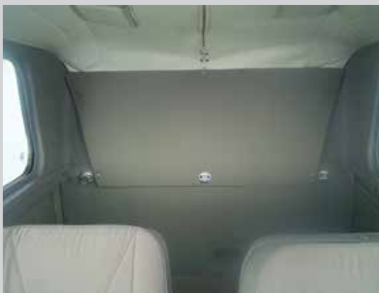
The rear firewall upholstery, installed over the rear firewall access panel for a clean look.
