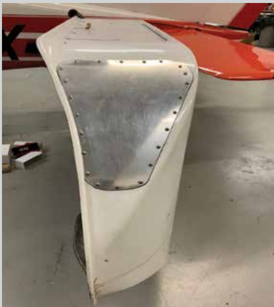
Skis, fishing rods, and other long items up to 86 inches long can be carried inside the Skymaster's cargo pod when an auxiliary door is installed.
