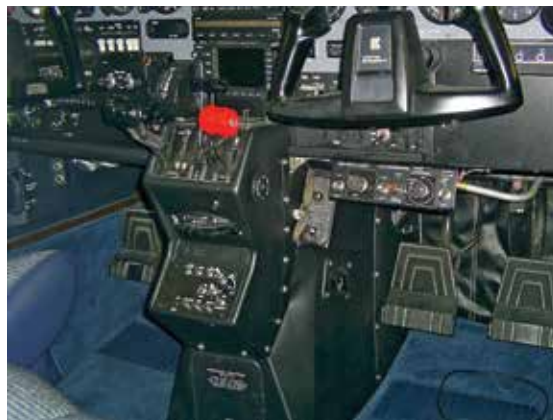
Aftermarket air conditioning controls are positioned under the co-pilot's yoke.
