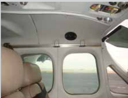
An air outlet over the pilot seat is standard for installation in later models, and optional for earlier models.
