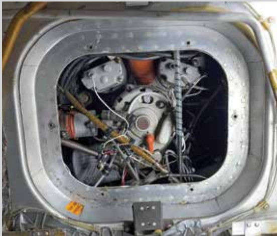
The factory-installed rear firewall door from a 1977 P337 Pressurized Skymaster.
