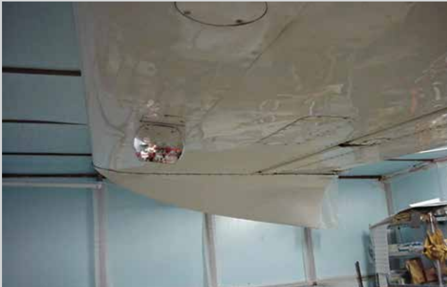
In addition to letting the pilot check the position of the landing gear, a convex mirror allows viewing all along the fuselage.
